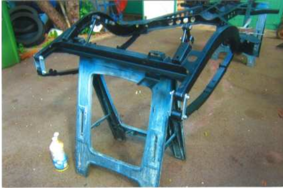
Chassis refinished—fitted rear springs
