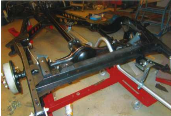
Rear chassis complete—propshaft & exhaust system
