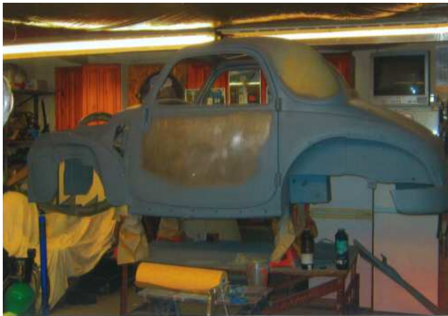
Body shell wings removed—stone chipped underneath awaiting paint prior to fitting to chassis
