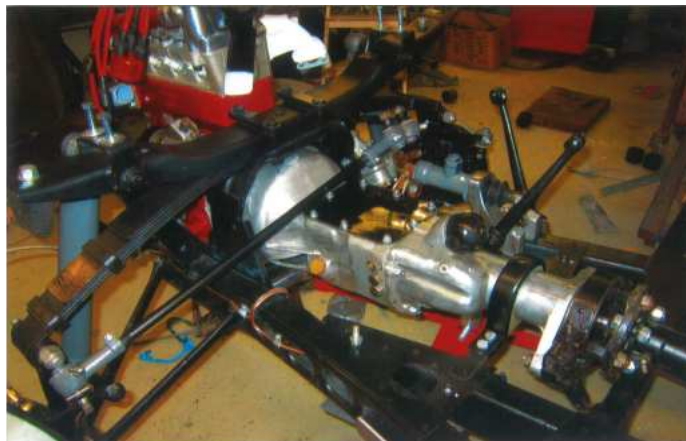
Rear view of gear box, master cylinder, peddles, Steering box and track-rods.
