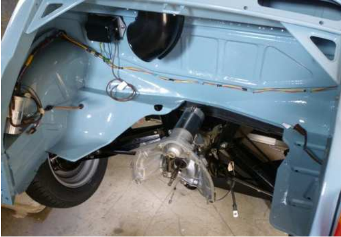
Gearbox fitted, but where's the engine ?
