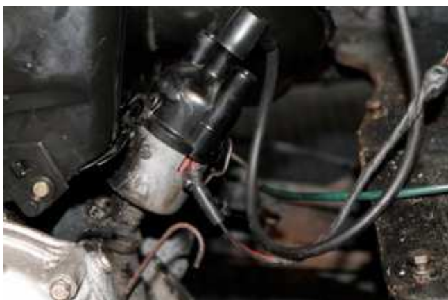
The old distributor with the loose cap
