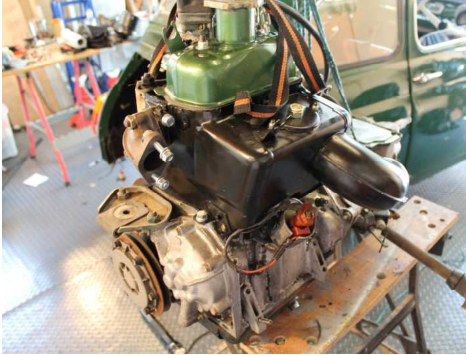
Engine out – Heater Casing fitted – Snazzy green Rocker Box fitted
