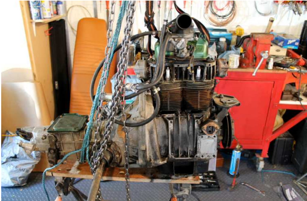
Cooling fan, fuel pump and distributor off
