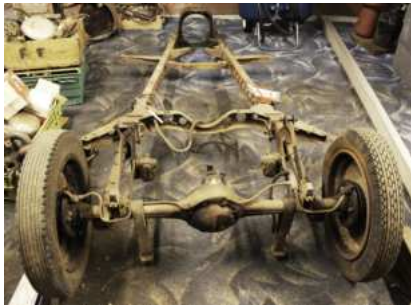
Chassis and rear axle and front axle being prepared
