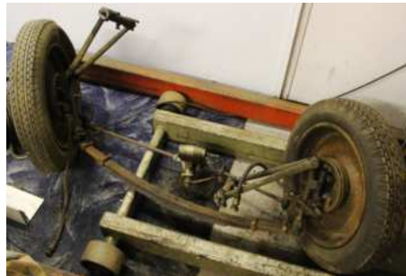
Chassis and rear axle and front axle being prepared
