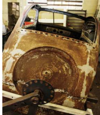
Topolino in a jig while welding takes place
