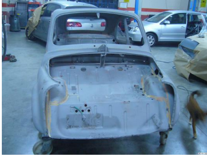
Feb 2009 blasted and ready for welding. I'm not sure if the cat helped!
