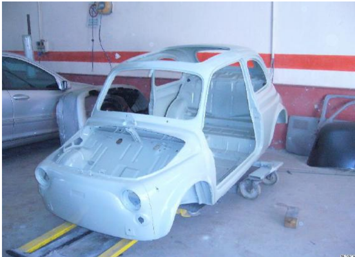
March 2009 Primed ready for paint
